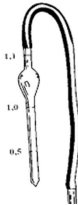
Figure 14. Special glass pipettes for WBC
